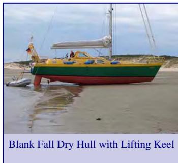
Blank Fall Dry Hull with Lifting Keel
